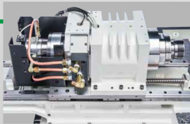
主軸夾頭用油壓缸 (適用於GO-325/GO-326) Hydraulic cylinder for main collet chuck (For GO-325/GO-326)
